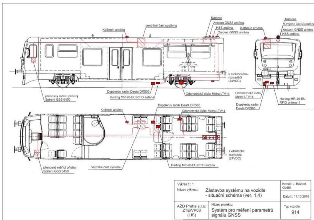
**Figure 6: Class 814 on-board installation**
