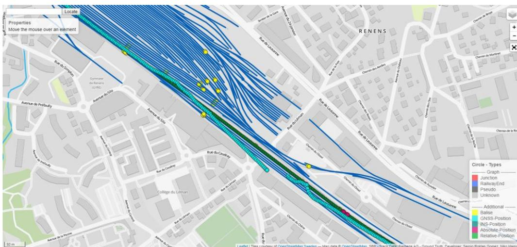
**Figure 28: Example 1 of GNSS data overlaid onto Ground Truth data**
