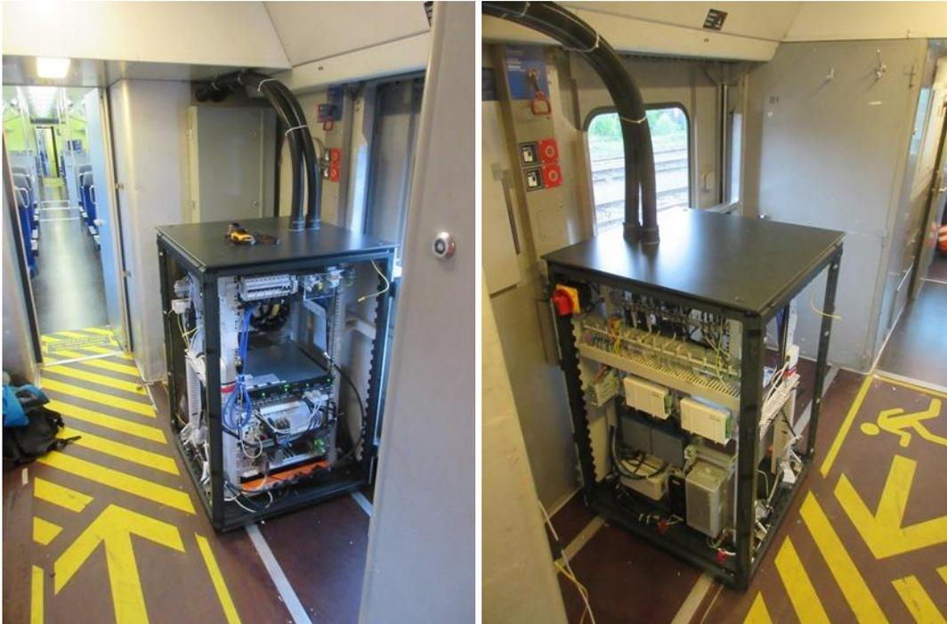
**Figure 18: Cabinet as installed, with doors removed**
