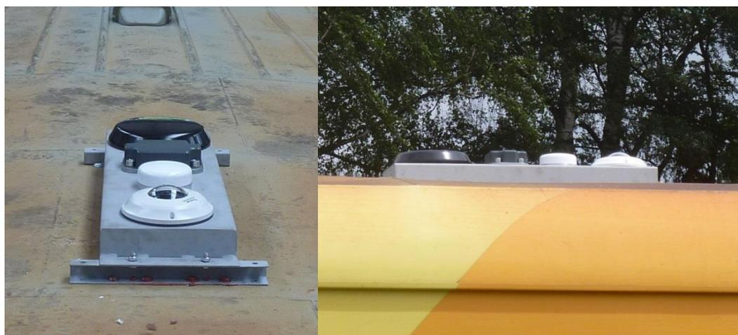
**Figure 7: Class 814 antenna and roof camera installation**
