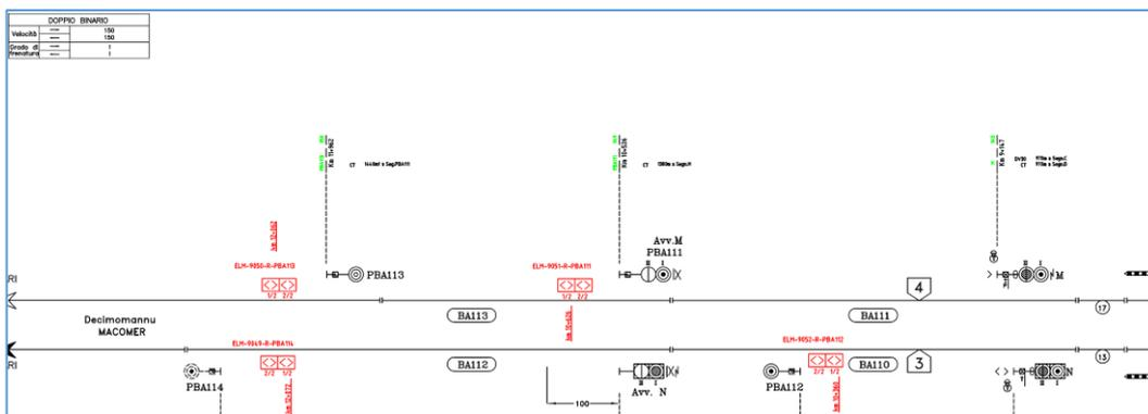
**Figure 42: Scheme plan with a small subset of Cagliari-San Gavino physical balises**
