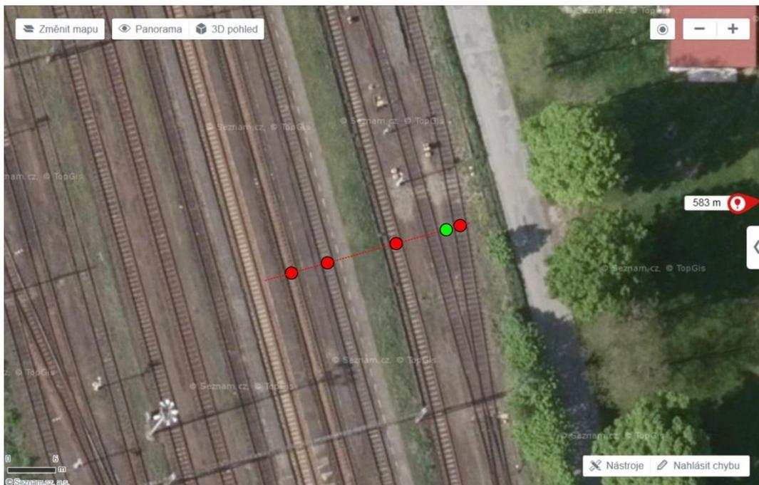
Figure 2: Placement of RF ID tags to distinguish tracks
