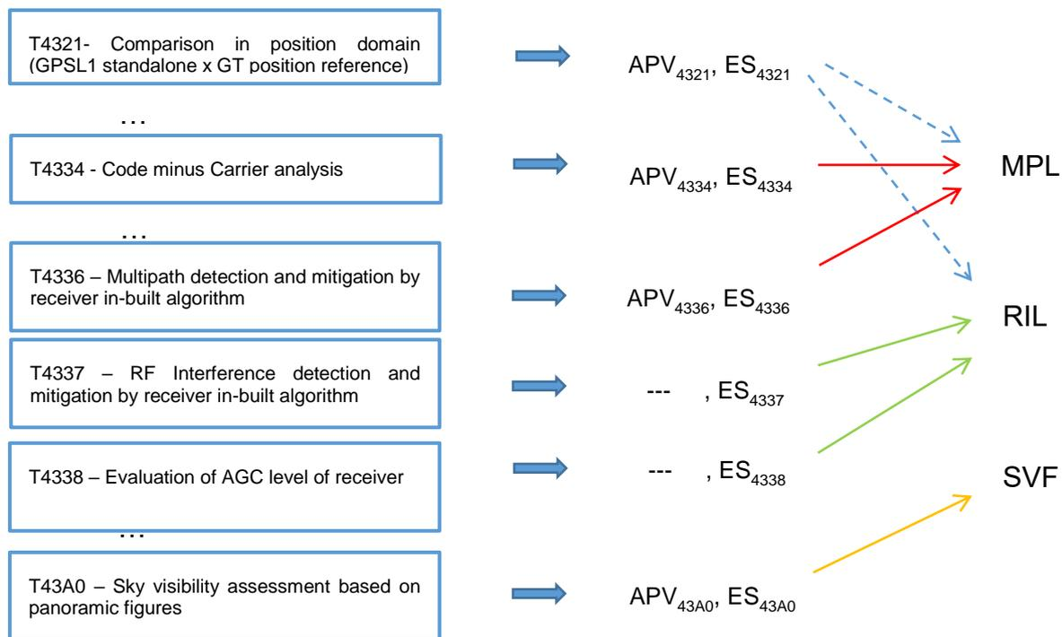
**Figure 50: Environment Characterisation Principle**
