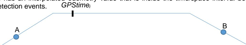
**Figure 22: Insight on a given odometry value (@*GPStime*) between two balises (A and B)**
