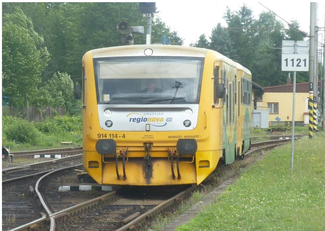
**Figure 5: Diesel multiple unit class 814 “Regionova”**
