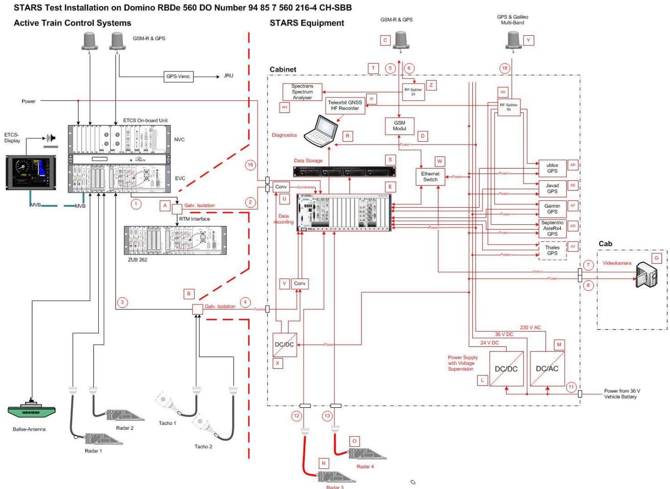
**Figure 15: Block Diagram of STARS Equipment**
