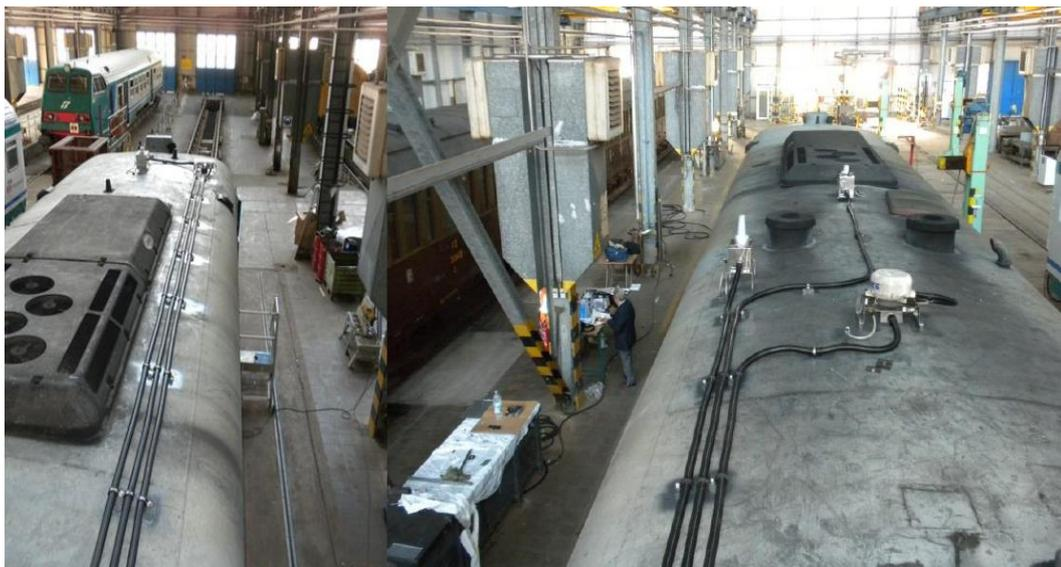
**Figure 12: GNSS antenna and cables installed on Cagliari-San Gavino train (ALn668)**
