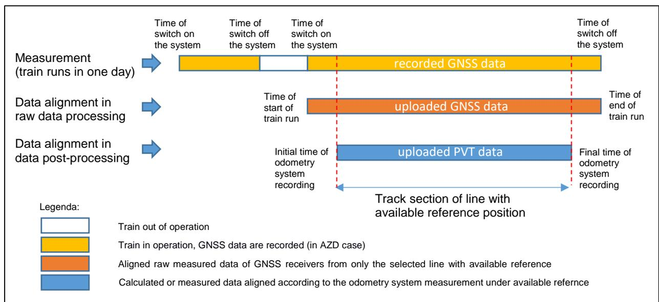
**Figure 48: Data Alignment Principle**
