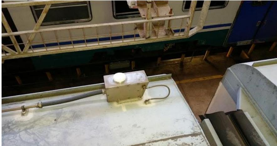
**Figure 13: GNSS antenna and cables installed on Pontremolese train (ALe642)**
