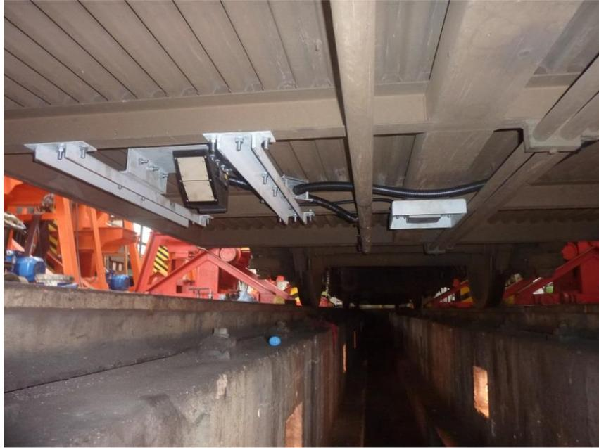
**Figure 10: Class 814 RF ID antenna and radar installation**
