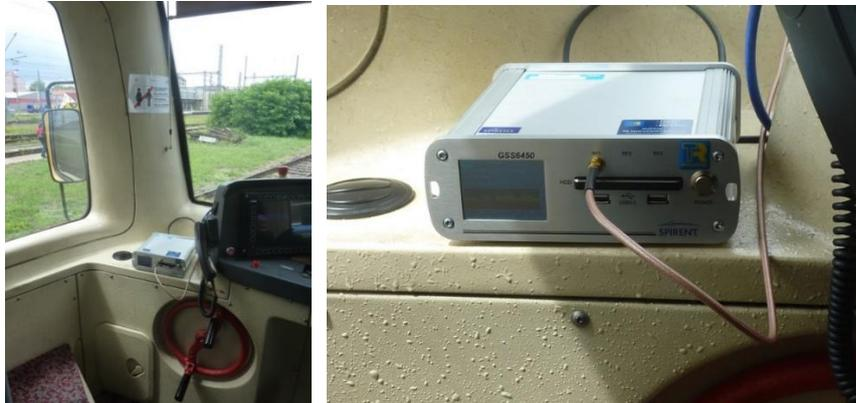
**Figure 8: Class 814 temporary installation of RPS Spirent**
